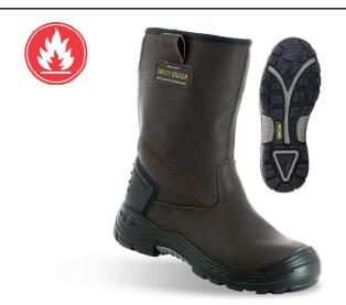
**Model description**: Leather boot, water repellent, brown, warm lining, antistatic, puncture resistant SJ Flex sole, shock proof, antislip, composite toe, S<sub>3</sub> PU/Rubber sole, HRO, CI.
